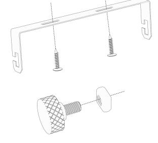
Push the square washer through the square shaped slot on the side track and slide the knob down the track to the desired mounting position.
