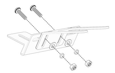
3. On the other end, insert (2) flat washers, (2) split lock washers, and (2) hex nuts to secure.
