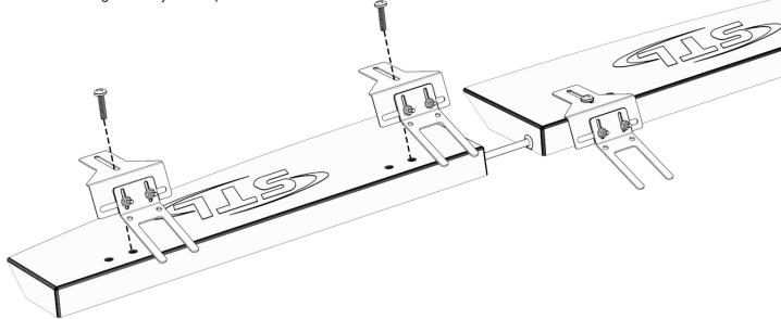
2. With all the assemblies now in place, adjust each visor bracket and base bracket to fit the vehicle. The flashback guard with the rubber stripping applied should be contacting the windshield. If the flashback guard is not touching the windshield you will need to use the other hole on the bottom of the Raptor and/or you will need to include spacers (see Page 10 for Spacer Installation).
