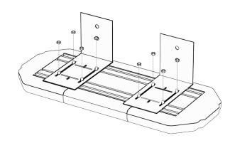
NOTE: IT IS VERY IMPORTANT TO POSITION THE BRACKET SO THAT THE LONGER PART OF BRACKET THAT ATTACHES TO THE LIGHTBAR POINTS TO THE REAR OF THE VEHICLE.
