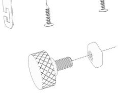
Push the square washer through the square shaped slot on the side track and slide the knob down the track to the desired mounting position.
