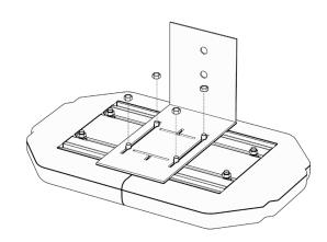
NOTE: IT IS VERY IMPORTANT TO POSITION THE BRACKET SO THAT THE LONGER PART OF BRACKET THAT ATTACHES TO THE LIGHTBAR POINTS TO THE REAR OF THE VEHICLE.
