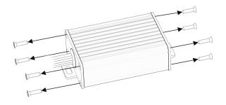
After removing all screws, the board can now be pulled out from its housing.
