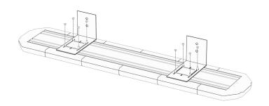
NOTE: IT IS VERY IMPORTANT TO POSITION THE BRACKET SO THAT THE LONGER PART OF BRACKET THAT ATTACHES TO THE LIGHTBAR POINTS TO THE REAR OF THE VEHICLE.
