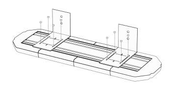
NOTE: IT IS VERY IMPORTANT TO POSITION THE BRACKET SO THAT THE LONGER PART OF BRACKET THAT ATTACHES TO THE LIGHTBAR POINTS TO THE REAR OF THE VEHICLE.
