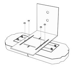
NOTE: IT IS VERY IMPORTANT TO POSITION THE BRACKET SO THAT THE LONGER PART OF BRACKET THAT ATTACHES TO THE LIGHTBAR POINTS TO THE REAR OF THE VEHICLE.
