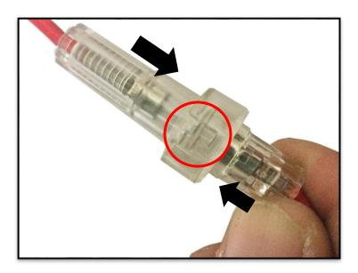
3. Once separated, remove fuse and attach to the extension cable top piece shown here
