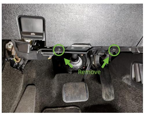
Remove the knee trim panel by pulling it toward the driver's seat. It is held in with five spring clips. It is easiest to start in the gap around the steering column and work your way around the rest of the panel (See below).
