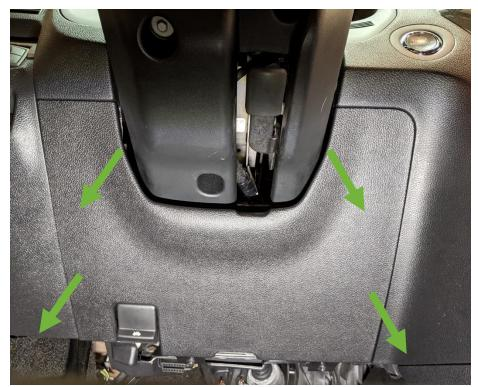
Remove the metal access plate by removing the four 10mm bolts pictured below.
