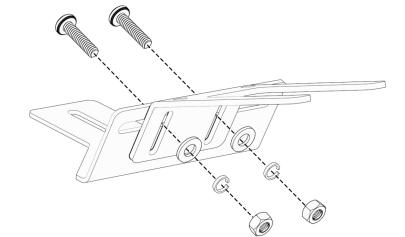
3. On the other end, insert (2) flat washers, (2) split lock washers, and (2) hex nuts to secure.
