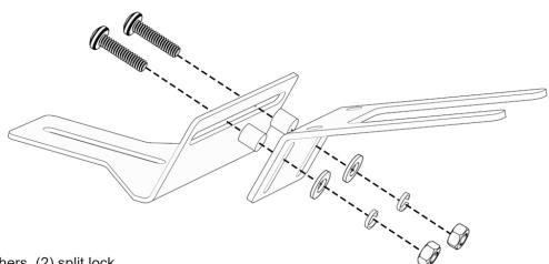
4. On the other end, insert (2) flat washers, (2) split lock washers, and (2) hex nuts to secure.
