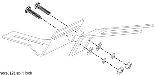
4. On the other end, insert (2) flat washers, (2) split lock washers, and (2) hex nuts to secure.
