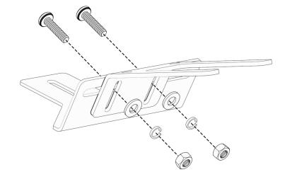
3. On the other end, insert (2) flat washers, (2) split lock washers, and (2) hex nuts to secure.
