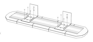
NOTE: IT IS VERY IMPORTANT TO POSITION THE BRACKET SO THAT THE LONGER PART OF BRACKET THAT ATTACHES TO THE LIGHTBAR POINTS TO THE REAR OF THE VEHICLE.
