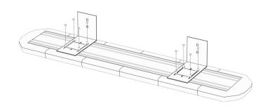
NOTE: IT IS VERY IMPORTANT TO POSITION THE BRACKET SO THAT THE LONGER PART OF BRACKET THAT ATTACHES TO THE LIGHTBAR POINTS TO THE REAR OF THE VEHICLE.
