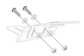
3. On the other end, insert (2) flat washers, (2) split lock washers, and (2) hex nuts to secure.
