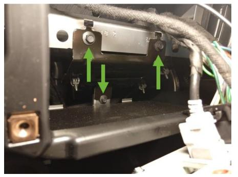
10. Disconnect the two connectors from the security gateway module and insert the connectors into the STE pass through connector. Ensure that both connectors are fully seated into the
