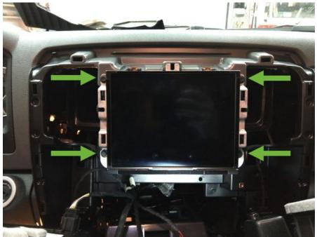
9. The security gateway module is mounted to a bracket directly behind the radio. Remove the three bolts that hold the bracket in place and pull the module out.
