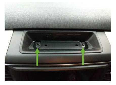
6. If the truck is equipped with a 115V outlet on the right side of the radio bezel you will need to remove one additional screw. Remove the rubber pad from the compartment above the outlet and remove the T20 screw located at the back.
