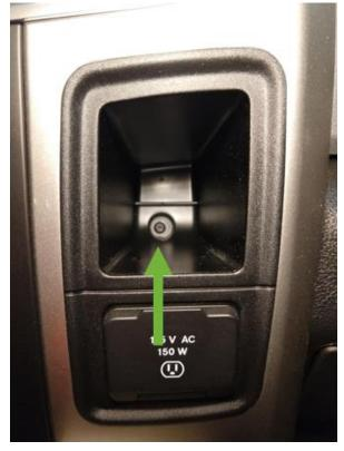
Pull the radio console bezel towards the rear of the vehicle to release the retaining clips.
