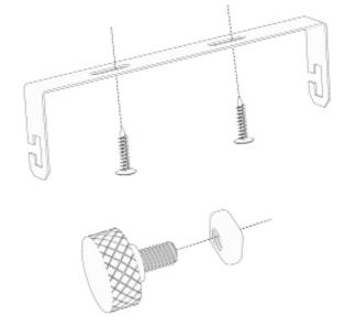
Push the square washer through the square shaped slot on the side track and slide the knob down the track to the desired mounting position.
