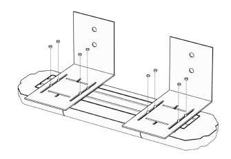
NOTE: IT IS VERY IMPORTANT TO POSITION THE BRACKET SO THAT THE LONGER PART OF BRACKET THAT ATTACHES TO THE LIGHTBAR POINTS TO THE REAR OF THE VEHICLE.
