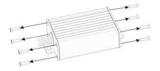
After removing all screws, the board can now be pulled out from its housing.
