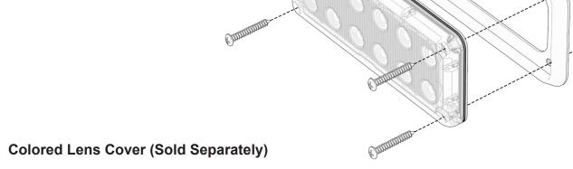
Unscrew all screws on the back of the unit and remove the stock lens cover.
