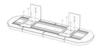
NOTE: IT IS VERY IMPORTANT TO POSITION THE BRACKET SO THAT THE LONGER PART OF BRACKET THAT ATTACHES TO THE LIGHTBAR POINTS TO THE REAR OF THE VEHICLE.
