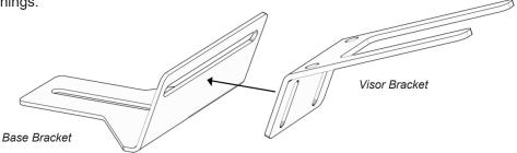
2. Insert (2) Phillips pan head screws through the base bracket opening.
