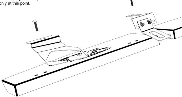
2. With all the assemblies now in place, adjust each visor bracket and base bracket to fit the vehicle. The flashback guard with the rubber stripping applied should be contacting the windshield. If the flashback guard is not touching the windshield you will need to use the other hole on the bottom of the Raptor and/or you will need to include spacers (see Page 10 for Spacer Installation).
