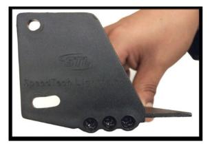
Replace End Cap Screws With the Longer Screws That Come With the Visor:
